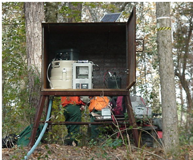
Figure 3. Monitoring station and rain gauges.
